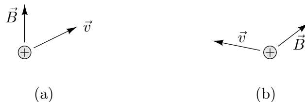
Figure 2.7. To apply the right-hand rule, place the velocity vector and the magnetic field vector tail-to-tail, as shown. Since this particle is positively charged, the magnetic force on it points out of the page in (a) and into the page in (b).
