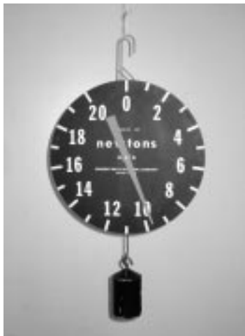
Figure 2.1. This spring scale measures the force being exerted to hold up the chunk of iron. Because this force just balances the downward pull of gravity, it is equal to the weight of the iron. The weight of this one-kilogram chunk of iron is 9.8 newtons.
