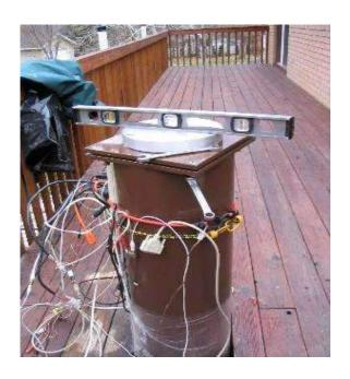
First (after getting the myriad wires out of the way) is leveling the thick aluminum plate that I made to sit on top of the pier. This plate was made very flat to provide a smooth surface for the MI-250 to sit on. I carefully leveled this plate using the adjusting bolts on the top plate of the pier.
