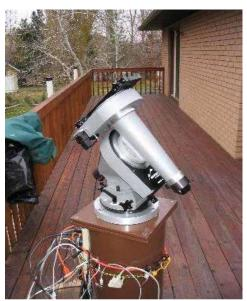
And the Dec housing with the dovetail base plate attached.
