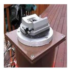
Next is to bolt on the MI-250 adapter plate and RA/Dec adjustment base.
