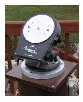
Then the RA housing drops onto the base.
