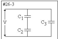
26-4. In the figure at right find the equivalent capacitance of the combination. Assume that  $C_1$  = 10.0  $\mu$ F,  $C_2$  = 5.00  $\mu$ F, and  $C_3$  = 4.00  $\mu$ F.
